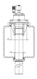
Note: Fix the valve body to the tank using the appropriate eyelets in the valve body
